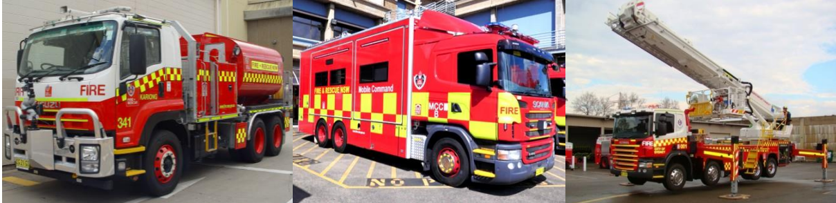
Figure 2 Specialist fire appliances: bulk water, command and aerial appliance (from l to r)
