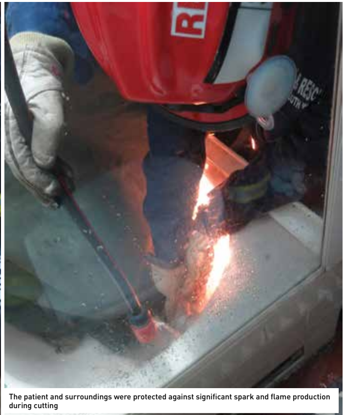
SO Rod Tabone operates an air powered angle grinder, fitted with a metal cutting disc, to cut through the bath tub. Firefighter Kamarah Pooley operates a garden hose, cooling the metal bath as it was being cut
