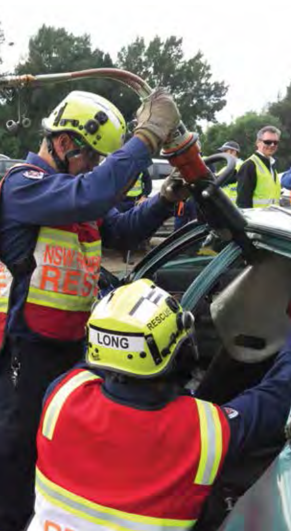
Rescue 59 cutting the C pillar in preparation for the forward roof flap
