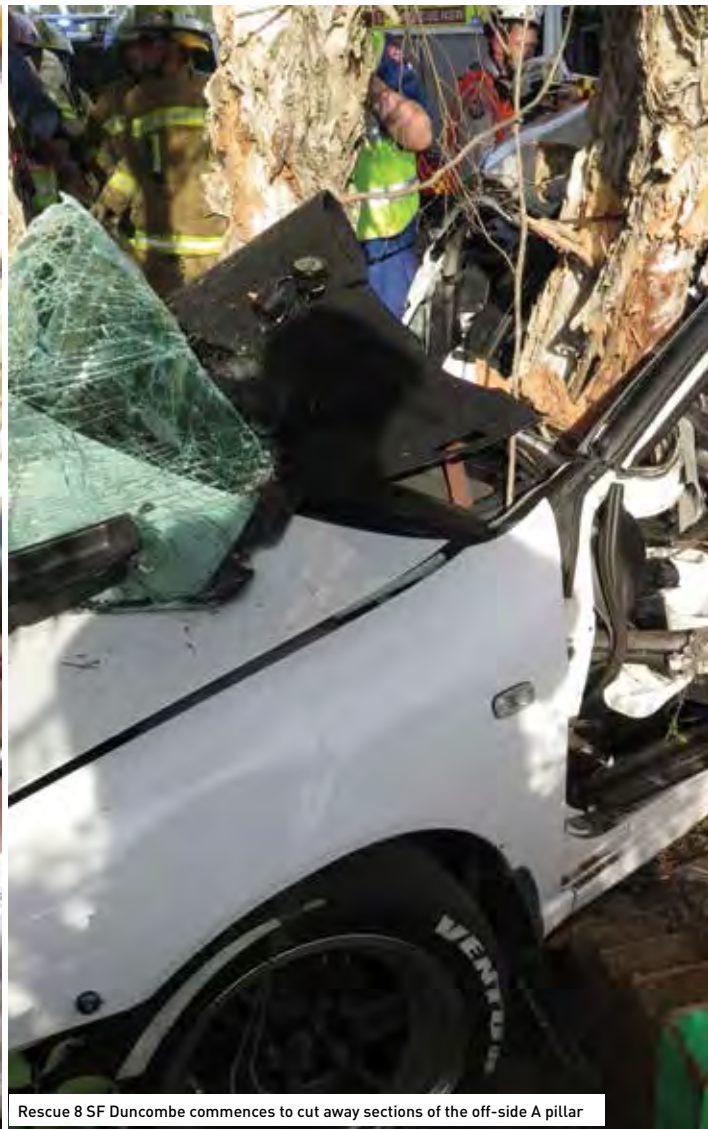
The floor-pan was pushed downwards with hydraulic spreaders, unfolding metal encasing the driver's lower limbs. A small hydraulic ram was then positioned to prevent the metal re-folding onto the patient. This process was repeated until the patient's lower limbs were completely removed from entrapment
