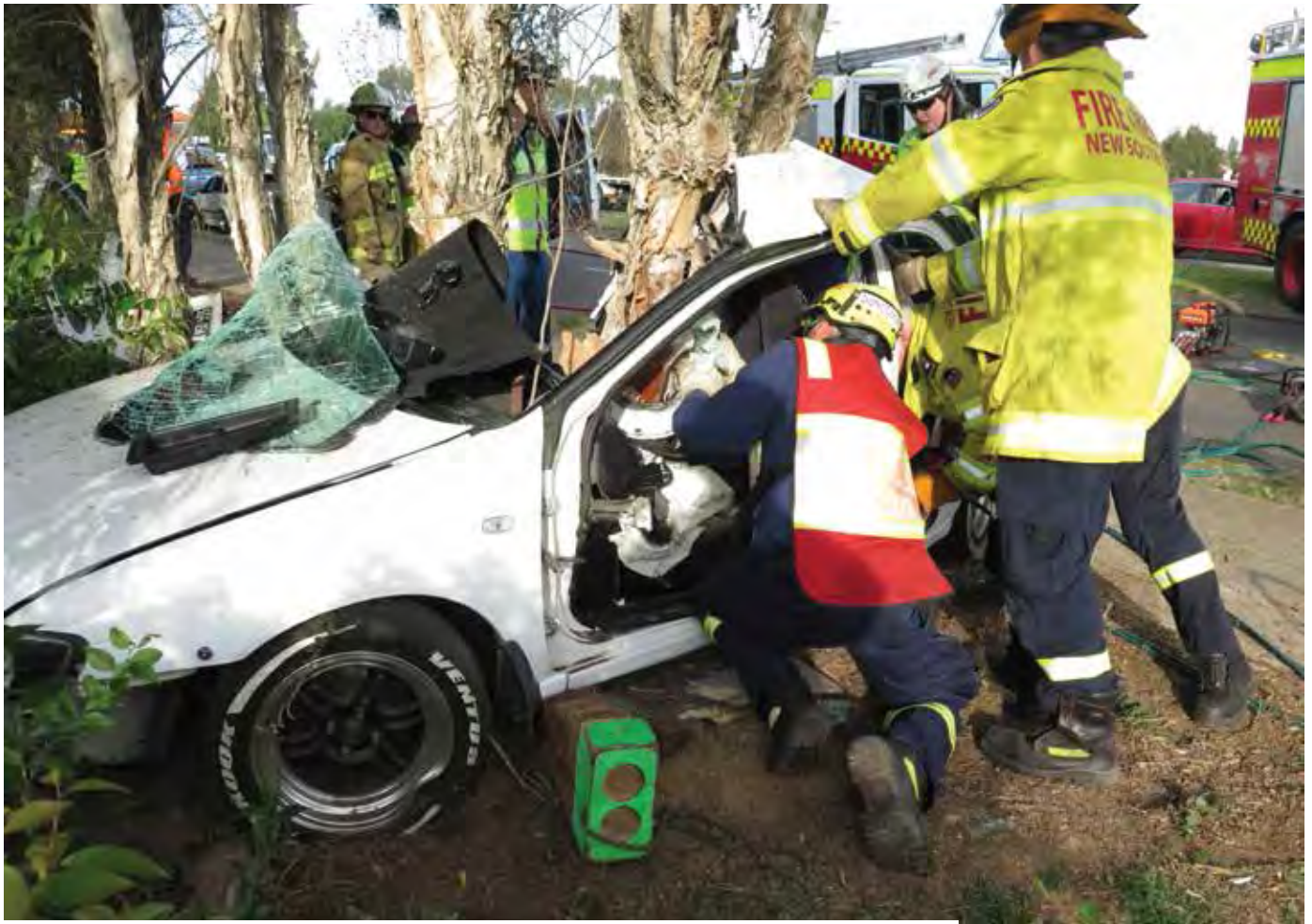
The scene shortly after firefighters commenced extrication; the off-side A pillar is visible (through the open door), wrapped around the tree
