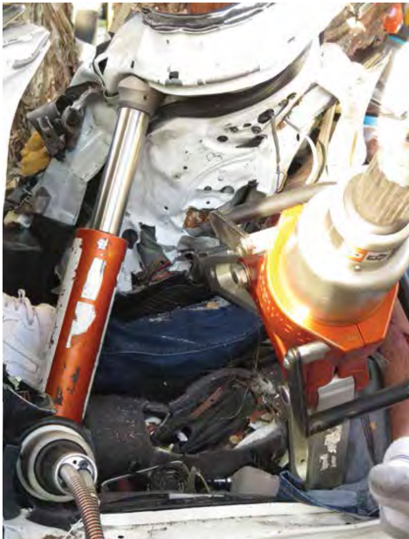
The floor-pan was pushed downwards with hydraulic spreaders, unfolding metal encasing the driver's lower limbs. A small hydraulic ram was then positioned to prevent the metal re-folding onto the patient. This process was repeated until the patient's lower limbs were completely removed from entrapment
