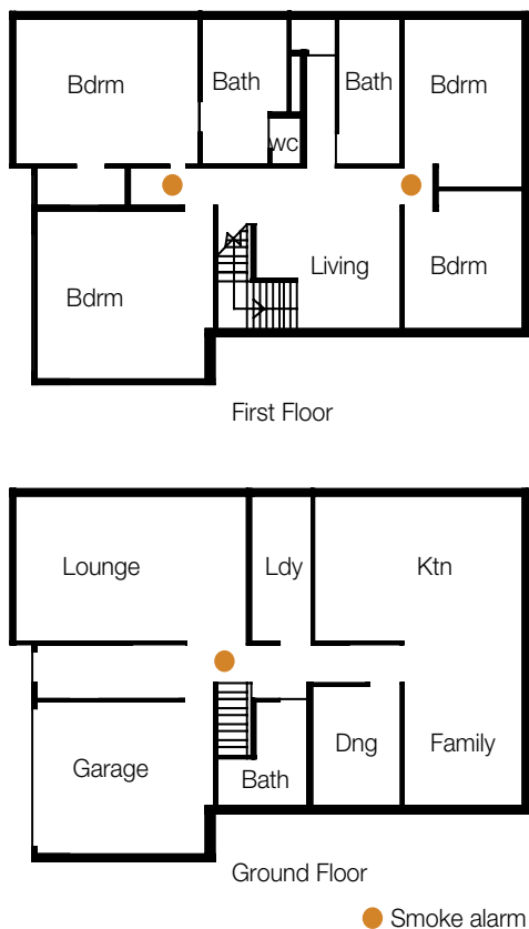
Diagram 3: Two storey dwelling showing smoke alarms in the storey containing bedrooms (first floor) and the storey not containing bedrooms (ground floor)
