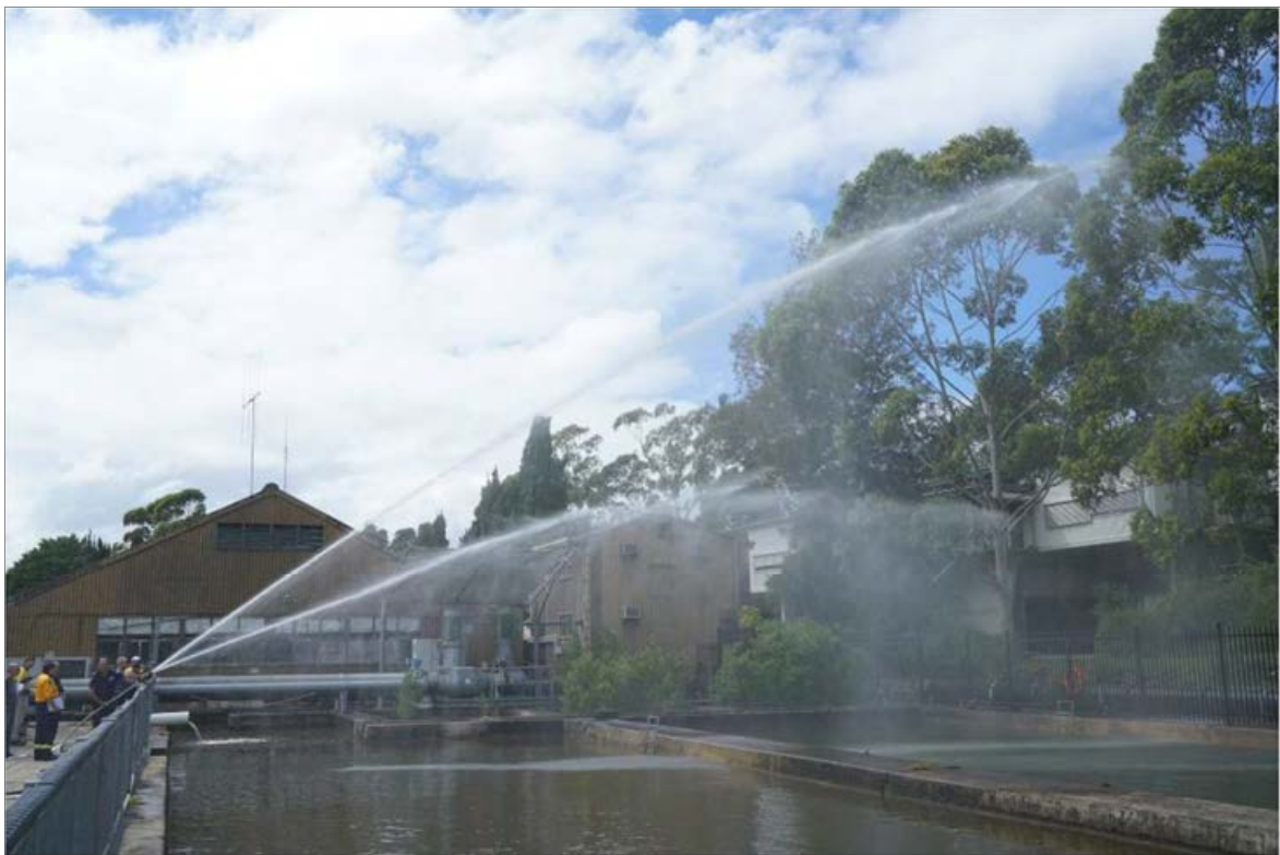
Figure 3-1: 10 l/s water stream- FRNSW Ø64mm Akron branch - single Ø64mm x 30m of lay-flat canvas hose
