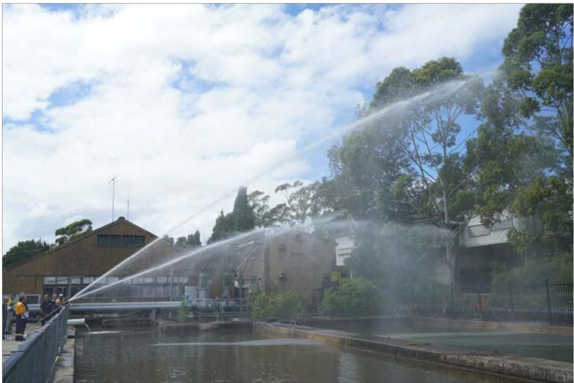
Photograph: 10 l/s water stream issuing from an FRNSW Ø65mm Akron branch via a single Ø64mm x 30m of lay-flat canvas hose
