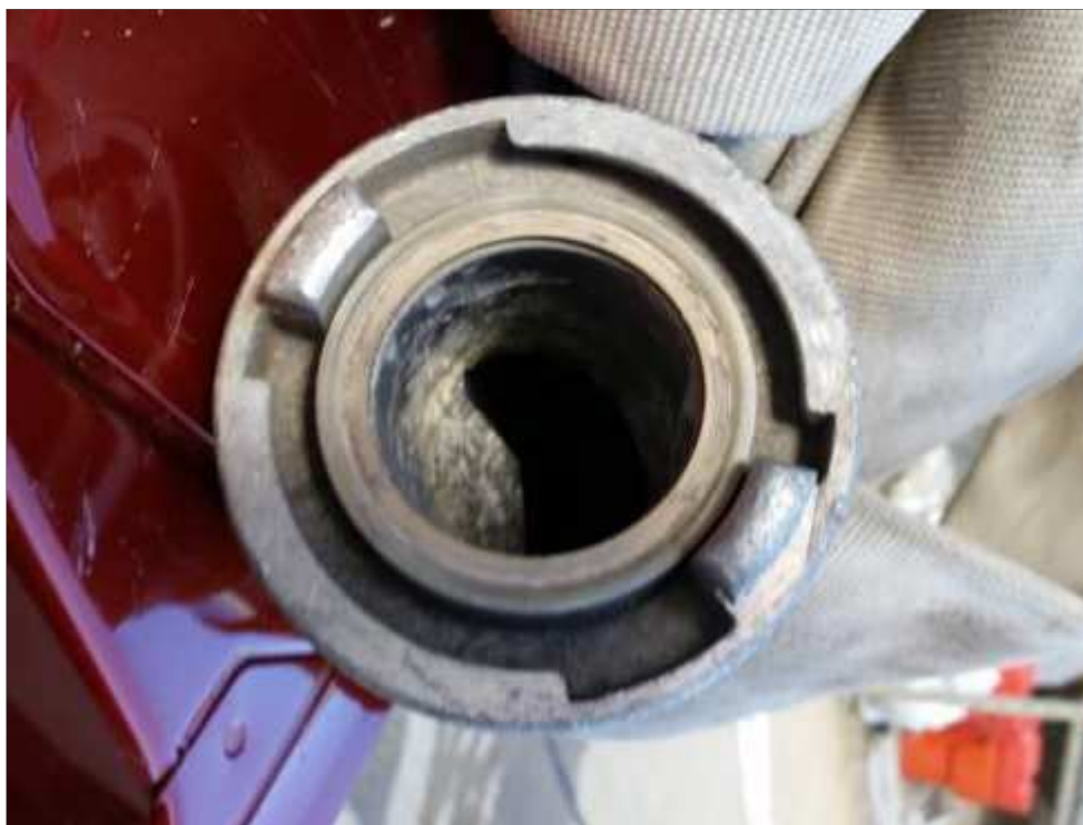
Figure B-2: Damaged hose coupling
