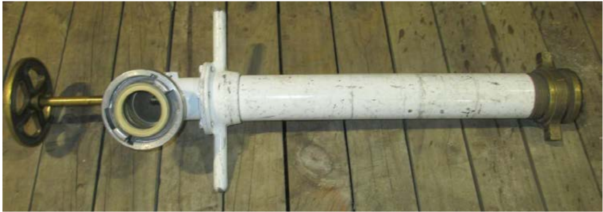
Figure A-5: Standpipe
