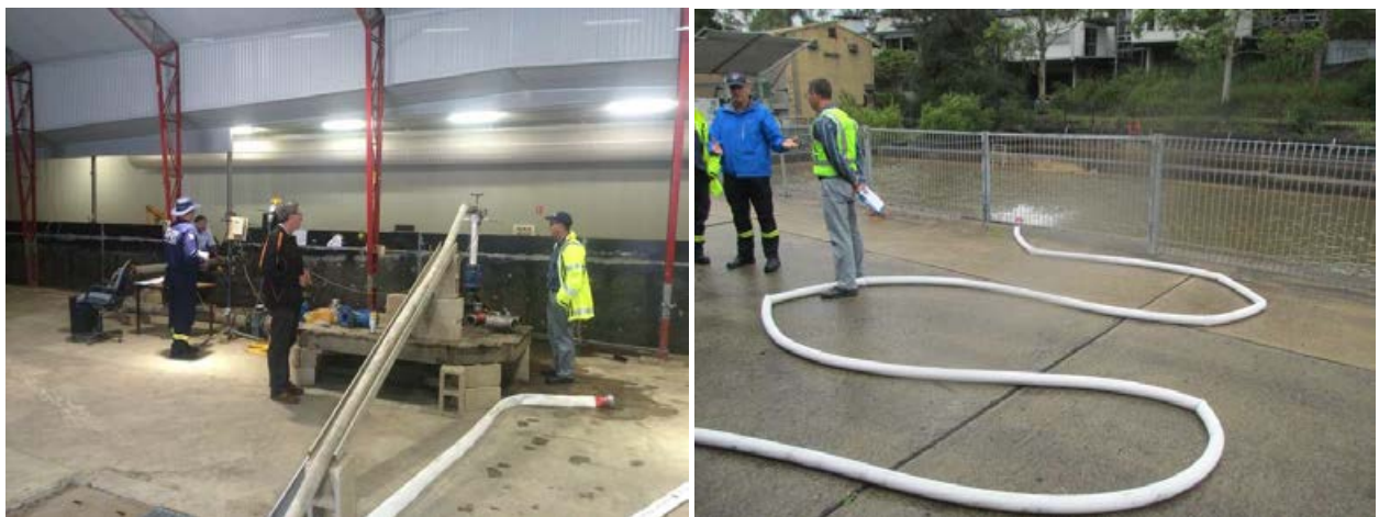
Figure 2-3: Hydrant supply to fire-fighting pumping appliance
