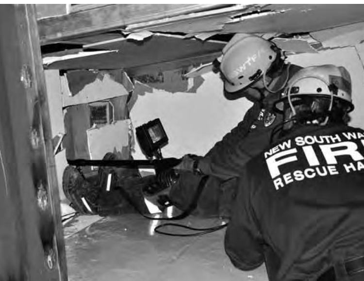
Using a search camera to search for trapped casualties inside a collapsed building
