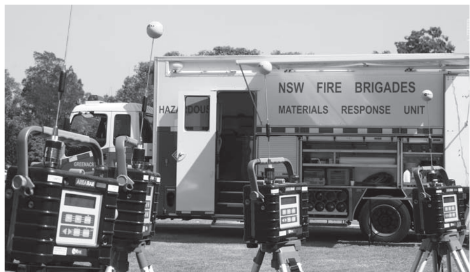
NSWFB's hazmat capabilities include atmospheric monitoring equipment, shown in foreground
